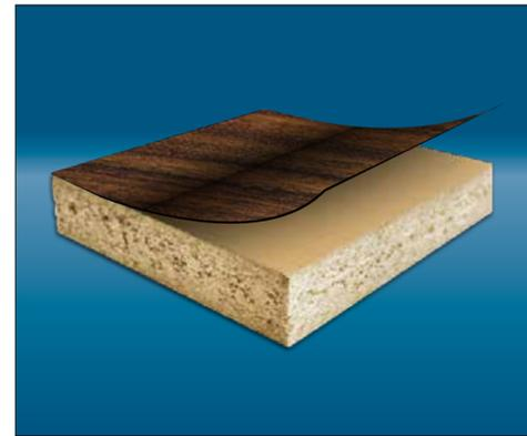
TFL (Thermally Fused Laminate) is made by fusing a resin-coated sheet of décor paper directly to a substrate. There is no kraft paper used in TFL, and the resulting panel is ready for fabricating.
