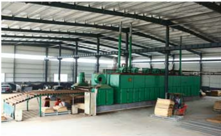
Veneers are conditioned by machine dryers to produce a core with a consistent moisture content (MC) ideal for lay-up, avoiding potential warp and instability within the platform.
