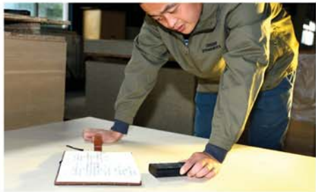
Core veneers then undergo a second more rigorous inspection for moisture content (MC) and thickness to ensure consistent sound cores.
