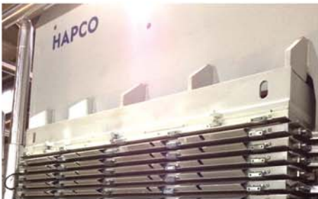
Composed core veneers are pressed in a multi-opening press using environmentally responsible and approved adhesives.
