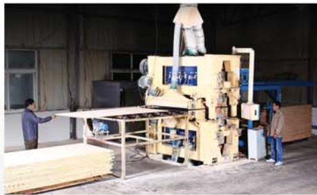
After pressing, cores are calibrated using a double head calibrating sander and are inspected again to ensure that they meet Dragon Ply's industry leading tolerances of +/- 0.3mm.
