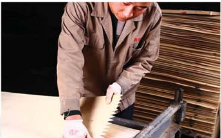
Precision finger joints or scarf joints ensure sound stable cores. Scarf jointing the outer most long-grain and machine composed outer crossbands reduces core overlaps, core voids and putty that may be visible on the finished panel as core shadow or telegraphing of imperfections. Imperfect cores are rejected for Dragon Ply.
